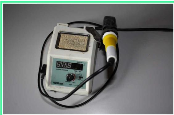
Soldering iron with a sponge to clean up the soldering tip.
